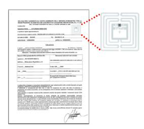
RFID tags integrated into paper are available as standard UHF EPC-GEN2 in short-range (21x21 mm) or medium-range format (93x23 mm).
