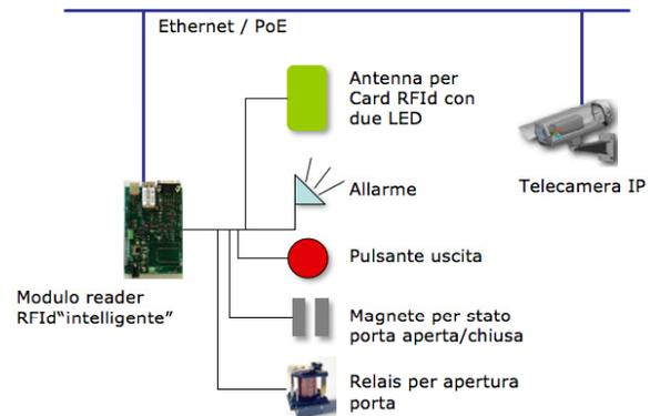
Diagram showing control of a door / gate
